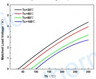
The chart for matched load voltage Vs T<sub>h</sub> under various T<sub>c</sub>
