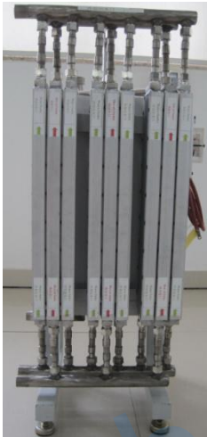
600W- 48VDC Output Thermoelectric Power Generator
